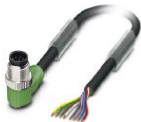
Sensor/actuator cable, 8-position, PVC, black RAL 9005, Plug angled M12, coding: A, on free cable end, cable length: 5 m
