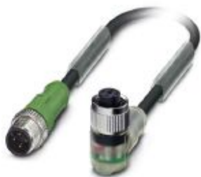
Sensor/actuator cable, 4-position, PVC, black RAL 9005, Plug straight M12, coding: A, on Socket angled M12, coding: A, with 3 LEDs, cable length: 3 m
