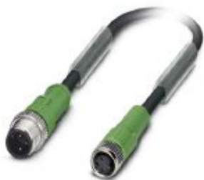
Sensor/actuator cable, 3-position, PVC, black RAL 9005, Plug straight M12, coding: A, on Socket straight M8, cable length: 0.6 m
