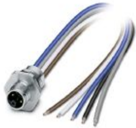
Flush-type connector, Power, 5-position, Plug, M12, L - Power, Front mounting, M16 x 1.5, Individual wires, cable length: 0.2 m, 2.50 mm 2 , PEX litz wire
