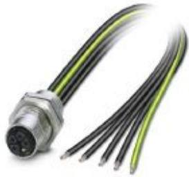
Flush-type connector, Power, 5-position, Socket, M12, K - Power, Rear mounting, M16 x 1.5, Individual wires, cable length: 0.2 m, 2.50 mm 2 , PEX litz wire
