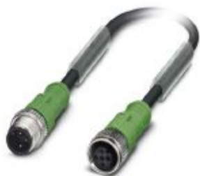
Sensor/actuator cable, 3-position, PVC, black RAL 9005, Plug straight M12, coding: A, on Socket straight M12, coding: A, cable length: 3 m
