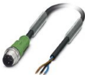
Sensor/actuator cable, 3-position, PVC, black RAL 9005, Plug straight M12, coding: A, on free cable end, cable length: 10 m
