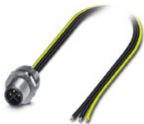
Flush-type connector, Power, 3-position, Plug, M12, S power, Front mounting, M16 x 1.5, Individual wires, cable length: 0.5 m, 1.31 mm 2 , UL/cUL stranded hook-up wire
