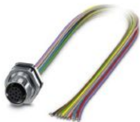
Flush-type connector, Universal, 12-position, Socket, M12, A-coded, Rear mounting, M16 x 1.5, Individual wires, cable length: 0.5 m, 0.14 mm 2 , TPE litz wire
