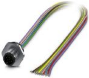
Flush-type connector, Universal, 12-position, Plug, M12, A-coded, Front mounting, M16 x 1.5, Individual wires, cable length: 0.5 m, 0.14 mm 2 , TPE litz wire
