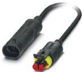
Sensor/actuator cable, 2-position, PUR halogen-free, black-gray RAL 7021, Plug straight Superseal Clip locking, on Socket straight Superseal Clip locking, cable length: 3 m
