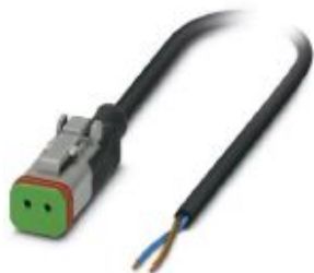
Sensor/actuator cable, 2-position, PUR halogen-free, black-gray RAL 7021, free cable end, on Socket straight DEUTSCH DT06-2S Clip locking, cable length: 1.5 m
