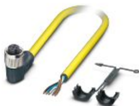
Sensor/actuator cable, 5-position, PVC, yellow, free cable end, on Socket angled M12, coding: A, cable length: 5 m
