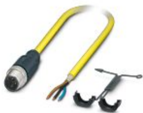
Sensor/actuator cable, 3-position, PVC, yellow, shielded, Plug straight M12, coding: A, on free cable end, cable length: 10 m
