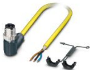
Sensor/actuator cable, 3-position, PVC, yellow, shielded, Plug angled M12, coding: A, on free cable end, cable length: 2 m
