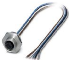
Sensor/actuator flush-type socket, 5-pos., M12, A-coded, front/screw mounting with M20 x 1.5 thread, with 0.5 m TPE litz wire, 5 x 0.34 mm 2 , brass version
