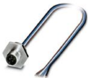
Sensor/actuator flush-type plug, 5-pos., M12, A-coded, front/screw mounting with M20 x 1.5 thread, with 0.5 m TPE litz wire, 5 x 0.34 mm 2 , brass housing
