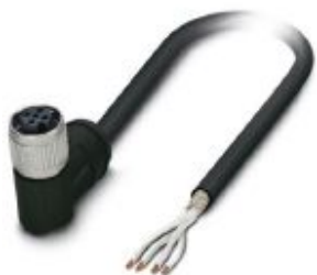
Sensor/actuator cable, 4-position, PE-X halogen-free, black, shielded, free cable end, on Socket angled M12 SPEEDCON, coding: A, cable length: 2 m, For railway applications
