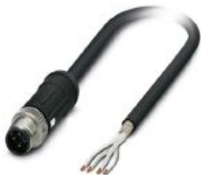
Sensor/actuator cable, 4-position, PE-X halogen-free, black, shielded, Plug straight M12 SPEEDCON, coding: A, on free cable end, cable length: 5 m, For railway applications
