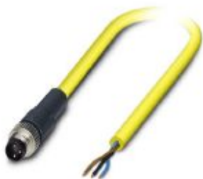
Sensor/actuator cable, 3-position, PVC, yellow, Plug straight M8, on free cable end, cable length: 5 m
