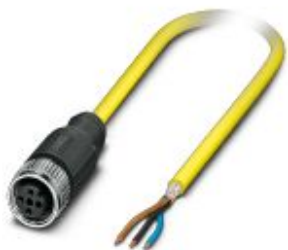
Sensor/actuator cable, 3-position, PVC, yellow, shielded, free cable end, on Socket straight M12, coding: A, cable length: 5 m
