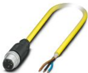
Sensor/actuator cable, 3-position, PVC, yellow, shielded, Plug straight M12, coding: A, on free cable end, cable length: 2 m
