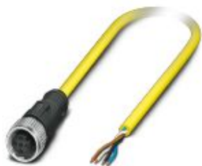
Sensor/actuator cable, 4-position, PVC, yellow, free cable end, on Socket straight M12, coding: A, cable length: 10 m
