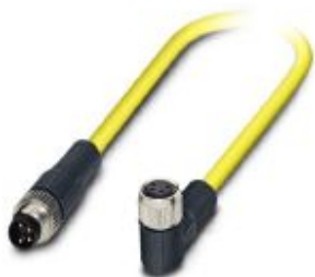
Sensor/actuator cable, 4-position, PVC, yellow, Plug straight M8, on Socket angled M8, cable length: 1.5 m
