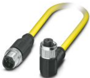
Sensor/actuator cable, 4-position, PVC, yellow, shielded, Plug straight M12, coding: A, on Socket angled M12, coding: A, cable length: 0.5 m
