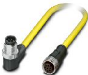
Sensor/actuator cable, 8-position, PVC, yellow, Plug angled M12, coding: A, on Socket straight M12, coding: A, cable length: 1.5 m
