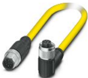
Sensor/actuator cable, 8-position, PVC, yellow, shielded, Plug straight M12, coding: A, on Socket angled M12, coding: A, cable length: 0.5 m
