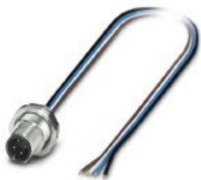
Sensor/actuator flush-type plug, 4-pos., M12, A-coded, rear/screw mounting with Pg9 thread, with 0.5 m TPE litz wire, 4 x 0.34 mm 2 , stainless steel design
