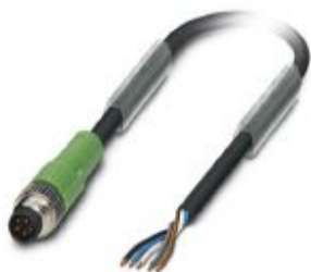
Sensor/actuator cable, 5-position, PUR halogen-free, black-gray RAL 7021, Plug straight M8, coding: B, on free cable end, cable length: 1.5 m
