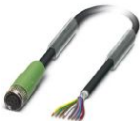
Sensor/actuator cable, 8-position, PUR halogen-free, black-gray RAL 7021, shielded, free cable end, on Socket straight M8, cable length: 5 m
