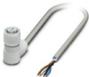
Sensor/actuator cable, 4-position, PP-EPDM halogen-free, gray RAL 7035, free cable end, on Socket angled M12, coding: A, with 3 LEDs, cable length: 5 m, Hygienic design, with plastic knurl
