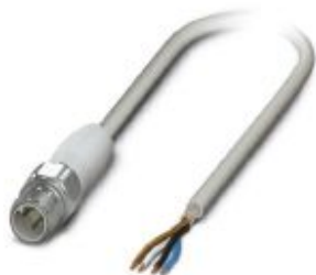
Sensor/actuator cable, 4-position, PP-EPDM halogen-free, gray RAL 7035, shielded, Plug straight M12, coding: A, on free cable end, cable length: 1.5 m, Hygienic design, with high-grade steel knurl
