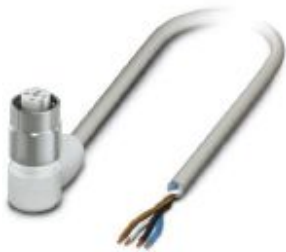
Sensor/actuator cable, 4-position, PP-EPDM halogen-free, gray RAL 7035, free cable end, on Socket angled M12, coding: A, with 3 LEDs, cable length: 10 m, Hygienic design, with high-grade steel knurl
