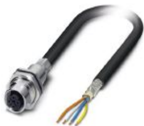
Assembled PROFINET cable, CAT5e, shielded, star quad, AWG 22 (7-wire), black, M12 flush-type socket, rear/screw mounting with M16 thread on free conductor end, length 2 m
