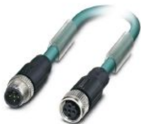
Bus system cable, PROFIBUS, 2-position, PUR/PVC, blue, shielded, Plug straight M12, coding: B, on Socket straight M12, coding: B, cable length: 5 m
