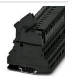
Fuse modular terminal block, fuse type: Glass / ceramics / ..., connection method: Screw connection, cross section:  $0.2 \text{ mm}^2$ -  $4 \text{ mm}^2$ , AWG: 24 - 12, nominal current: 32 A, nom. voltage: 400 V, width: 8.2 mm, fuse type: G /  $6.3 \times 32$ , mounting type: NS 35/7.5, NS 35/15, NS 32, color: black
