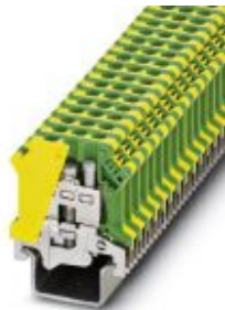
Ground terminal block with screw connection, cross section: 0.5 ... 6 mm 2 , AWG: 20 ... 8, width: 8.2 mm, color: green...yellow
