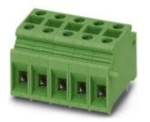
PCB terminal block, nominal current: 76 A, nom. voltage: 320 V, pitch: 10 mm, number of positions: 2, connection method: Screw connection with tension sleeve, mounting: Wave soldering, conductor/PCB connection direction: 0 $^{\circ}$ , color: green
