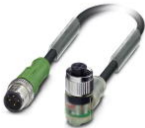
Sensor/actuator cable, 4-position, Variable cable type, Plug straight M12, A-coded, on Socket angled M12, A-coded, with 3 LEDs, cable length: Free input (0.2 ... 40.0 m)
