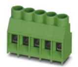
PCB terminal block, nominal current: 32 A, nom. voltage: 630 V, pitch: 6.35 mm, number of positions: 2, connection method: Screw connection with tension sleeve, mounting: Wave soldering, color: green
