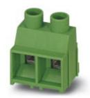
PCB terminal block, nominal current: 32 A, nom. voltage: 1000 V, pitch: 9.52 mm, number of positions: 2, connection method: Screw connection with tension sleeve, mounting: Wave soldering, conductor/PCB connection direction: 0 °, color: green
