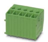
PCB terminal block, nominal current: 32 A, nom. voltage: 630 V, pitch: 7.62 mm, number of positions: 5, connection method: Front screw connection, mounting: Wave soldering, conductor/PCB connection direction: 90 °, color: green
