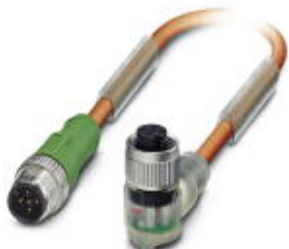
Sensor/actuator cable, 5-position, PUR halogen-free, irradiated, orange RAL 2003, Plug straight M12, A-coded, on Socket angled M12, A-coded, with 3 LEDs, cable length: 1 m, Customer-specific version
