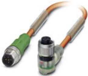
Sensor/actuator cable, 5-position, PUR halogen-free, irradiated, orange RAL 2003, Plug straight M12, A-coded, on Socket angled M12, A-coded, with 3 LEDs, cable length: 0.6 m, Customer-specific version
