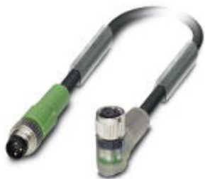
Sensor/actuator cable, 3-position, PUR halogen-free, black-gray RAL 7021, Plug straight M8, on Socket angled M8, with 2 LEDs, cable length: 1 m
