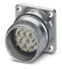
Device connector for front wall, straight, shielded: yes, Screw locking, M23, Radial O-ring, 4x Ø 3.2
