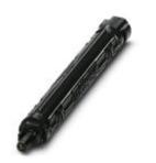
Fuse connector for protecting modules and devices in photovoltaic systems, black, SUNCLIX pin connector pattern, 1500 V/20 A, IP68 (24 h/2 m)
