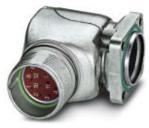
Device connector, front mounting, angled rotatable, Screw locking, M23, number of positions: 12, type of contact: Socket, Crimp connection, Axial O-ring, 4x  $\emptyset$  3.2, shielded: yes, flange dimensions: 28 mm x 28 mm
