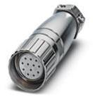
Cable connector, with Pg9 connection thread, straight, shielded: yes, Screw locking, M23, No. of pos.: 12, type of contact: Socket, Solder connection
