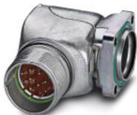
Device connector, front mounting, angled fixed, Screw locking, M23, number of positions: 16, type of contact: Pin, Crimp connection, Axial O-ring, 4x Ø 3.2, shielded: yes, flange dimensions: 26 mm x 26 mm
